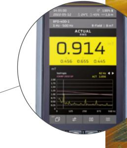
Unlike electric fields, magnetic fields are not easily shielded. The new H field probes from Narda measure magnetic fields omnidirectionally and can easily be precisely positioned, thanks to the geometric arrangement of their coils.
