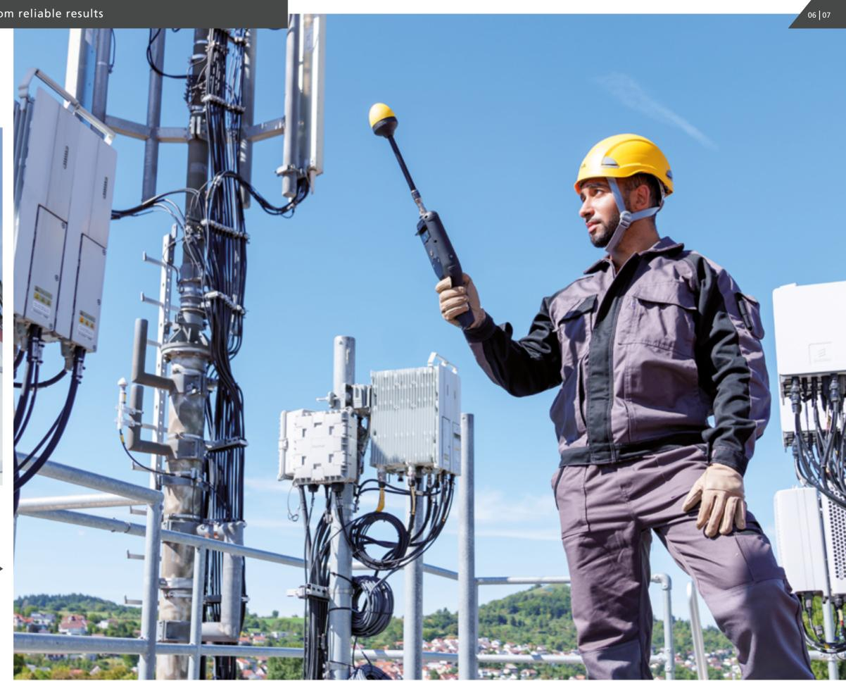
Narda FieldMan – Detecting and measuring electromagnetic fields
