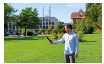
The ultrasonic distance meter precisely measures the height above ground where the FieldMan is being operated. The measurement is accurate to within one centimeter, with a capture angle of 15 degrees and a range of 25 cm to 400 cm. The measurement units can be set to meters, inches, feet or yards. Separate measurement with a ruler is therefore no longer necessary.
