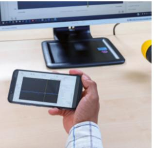
The WiFi / Bluetooth interface enables remote control of the FieldMan via the optional smartphone app. In this way, you can create photos and videos that can be added to the measurement data.
