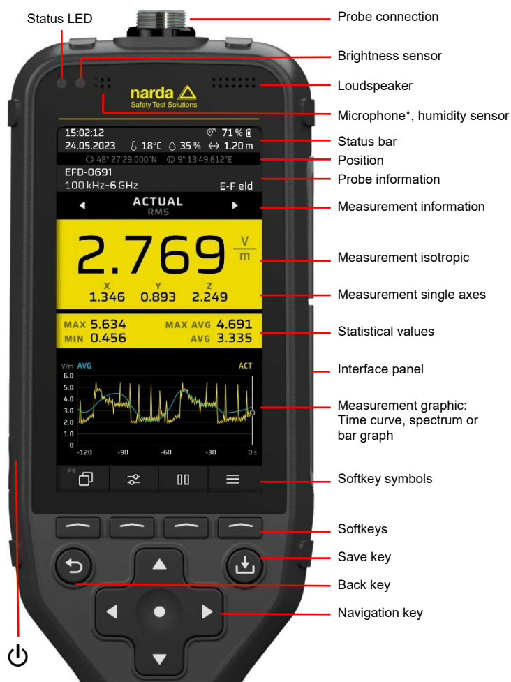
Fig. 2. FieldMan display and controls
