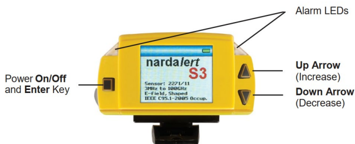
Fig. 1. Top view with display and controls
