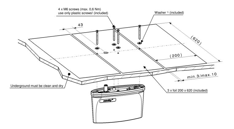
This drawing can be used as drilling template.
